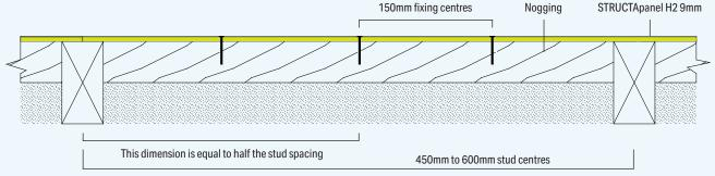
Any additional noggings must be evenly spaced across the wall height. Two noggings are required for walls that are 2440mm or 2745mm high. For walls that are 3050mm high, three noggings are required. STRUCApanel H2 9mm must be fixed to noggings at a maximum of 150mm centres.
